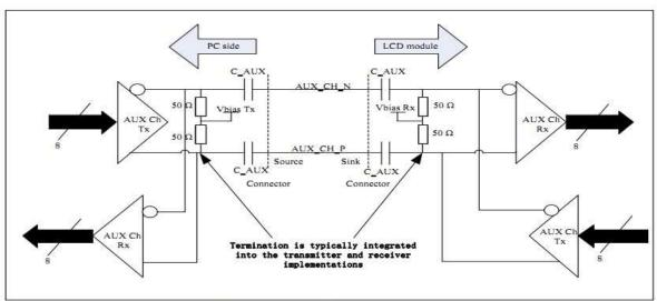
Fig.4-2-3 AUX Link differential pair
