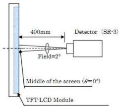
Fig.9-2 Measurement of Contrast, Luminance, Chromaticity, White variation, Crosstalk and Color temperature variation.
