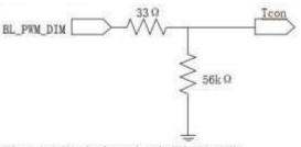
Fig.4-1-3 Equivalent circuit (Pin No.23)
