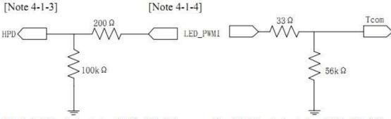
Fig.4-1-1 Equivalent circuit (Pin No.17)
