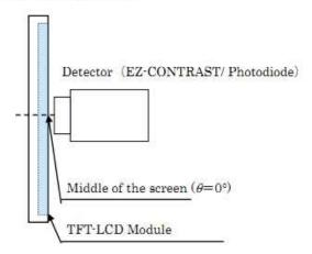
[Note 9-: Fig.9-1 Measurement of Viewing angle range and Response time.
